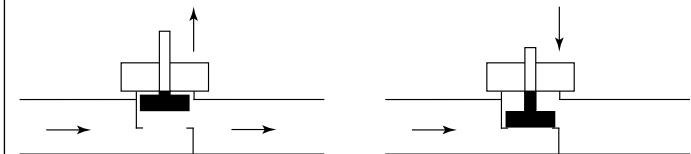
Figure 3 Left: Valve is open when the valve stem is extended. Right: Valve is closed when the valve stem is pushed into the valve.
