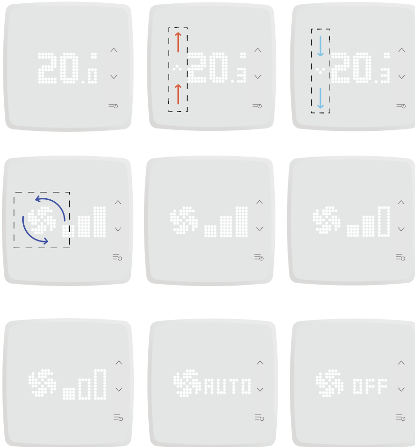
Figure 2-3 Indications in the controller display 1
